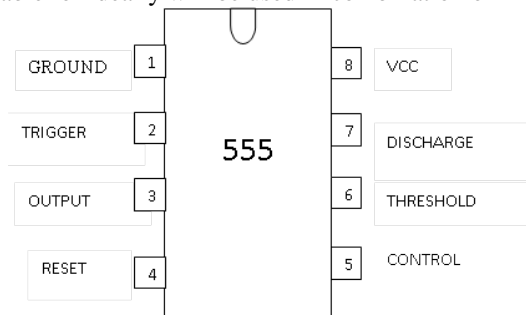
Fig. 2: Pin out diagram of TIMER IC555
