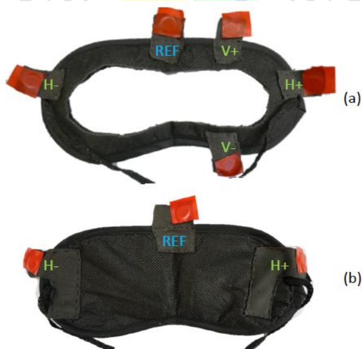
Fig. 7.1: Sleep masks with graphene-based nylon sensors sewn in, showing the view from back of the mask.
